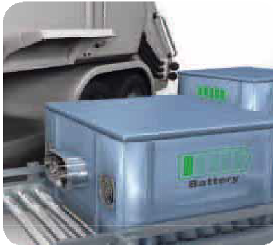
The empty battery is removed.
