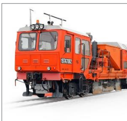
RB Ballast Distributor
