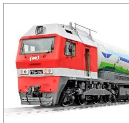
GT1h Mainline Gas Turbine Locomotive
