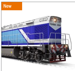
TGM8km Removing Switcher with Hydraulic Drive
